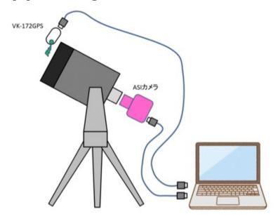
GPS synchronization VK-172GPS is commercially priced at about 1000 yen (JPN). The VK-172GPS emits extremely accurate (uncertainty is less than microsecond) second signals synchronized with GPS by green LED.
